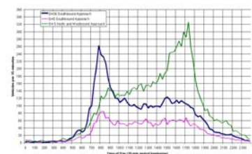
Figure 3: Average weekly 15 minute traffic volumes recorded on each approach to the roundabout
