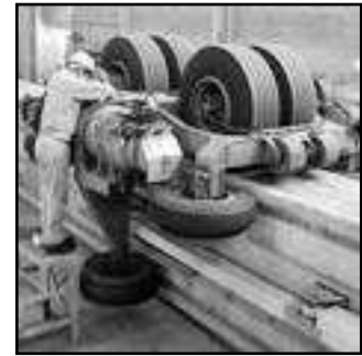
Figure 13: ALWEG running gear
