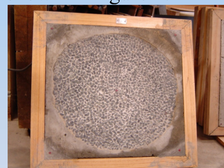
Step 1: Preparing an aggregate sample to test
