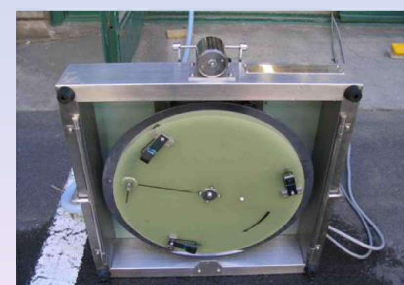
The Dynamic Friction Tester and Rubber sliders
