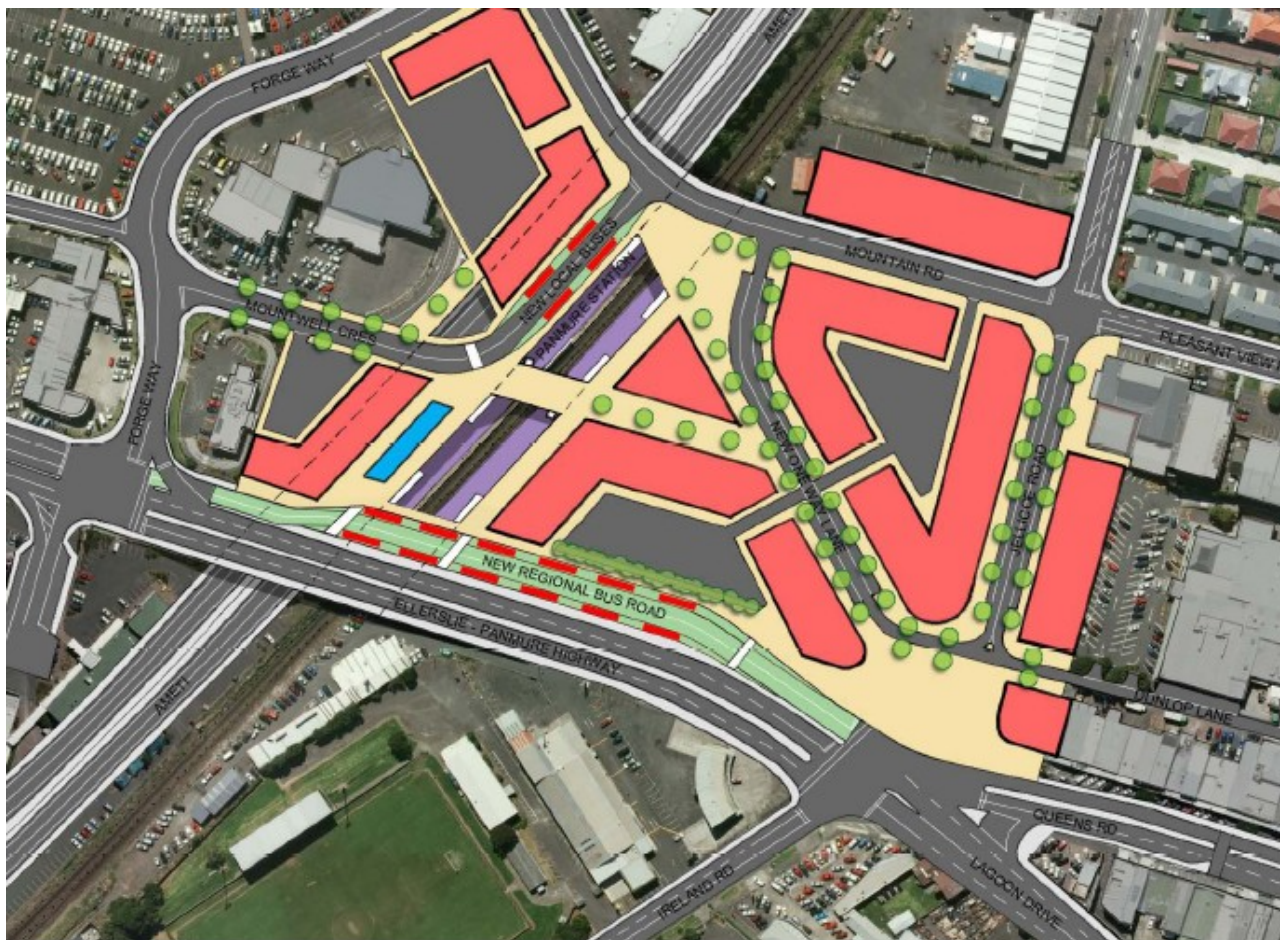
Figure 9: Panmure Interchange – Segregated Busway #2
