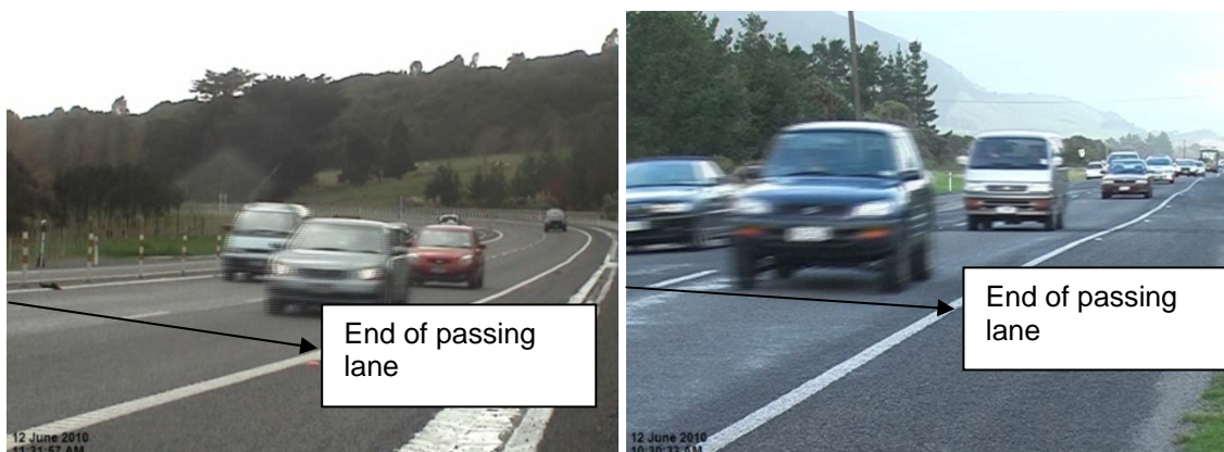
Figure 3. Examples of Level 2 merging behaviour at Sites 9 (left) and 4 (right). In each example, some action would need to be taken by at least one of the motorists in order to maintain a safe separation between vehicles
