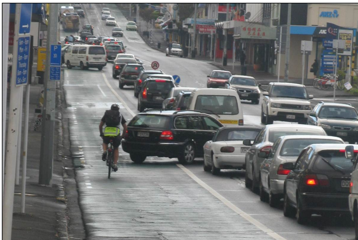
Figure 2 - Example of the multiple turning movements across bus lanes and the relative size of a cyclist within the lane
