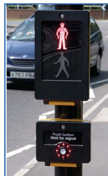
Figure 6: Nearside signal display (UK)
