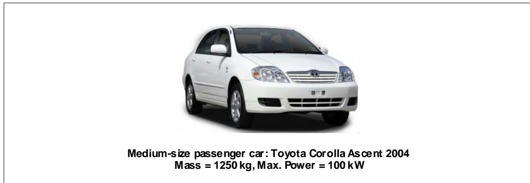
Figure 2 – The test vehicle used for fuel consumption model calibration results reported in this paper
