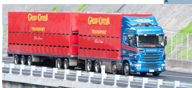
50MAX axle configuration
