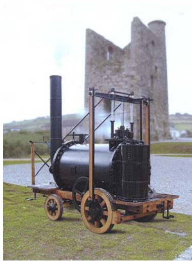
Contrast: Newcomen/Watt use of low pressure steam in a beam engine and Trevithick's first essay into high pressure steam.
