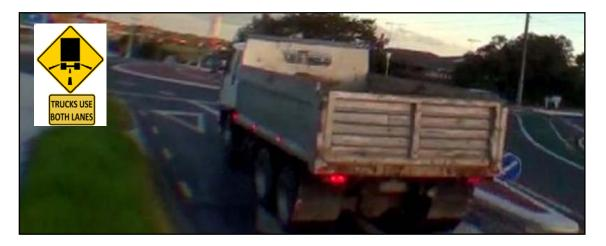
Figure 1: Truck straddling the two narrow lanes on approach to a C-Roundabout. Although fairly intuitive to drivers, advance warning signs are considered desirable with an example used shown inset.
