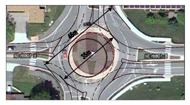
Figure 2: A C-Roundabout alignment atop a typical dual-lane layout from the United States, which is similar to Austroads in terms of space requirements.
