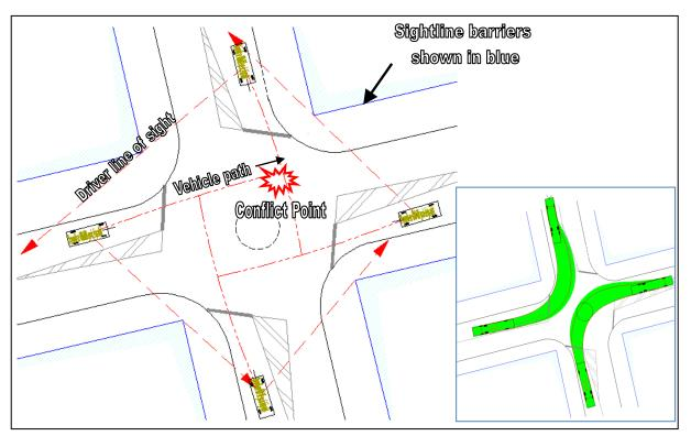
Figure 4: Concept drawing for a single-lane roundabout (outside diameter approx. 20m or smaller) using sight line restrictions with low mountable or flush central island. Inset is shown large bus tracking.
