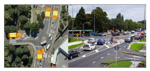
Figure 3: 'Directional' platforms were installed in 2010 at the Vitasovich Ave / Edsel St roundabout in Auckland (although not all platforms were constructed to the specified heights).
