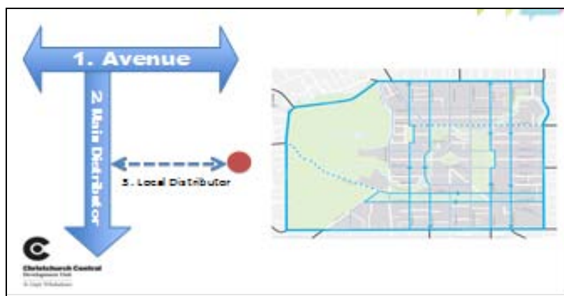
Figure 13. AAC three tier approach for the general traffic network hierarchy
