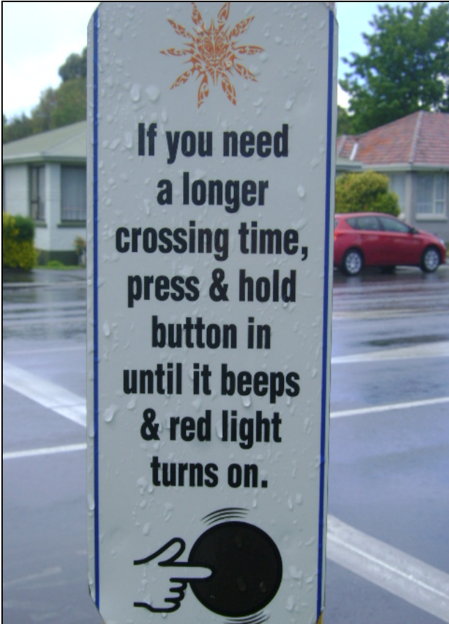
Figure 3 - DPCS Pole mounted metal signage advising pedestrians that a longer crossing time can be chosen, if they need it, by holding the button in until it beeps and red LED activates
