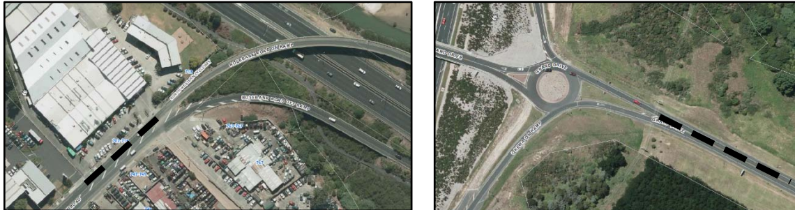
Figure 28: Local road transitions to on/off ramps should have ATP applied where indicated
