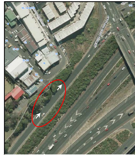
Figure 19: Supplementary direction arrows marked to reinforce direction of travel
