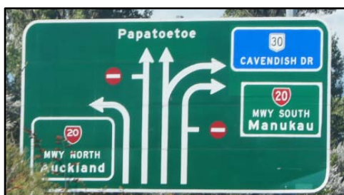
Figure 16: Lane assignment diagrammatic sign – Too much information to absorb quickly, & in this case too far to the left of the carriageway for right turners.
