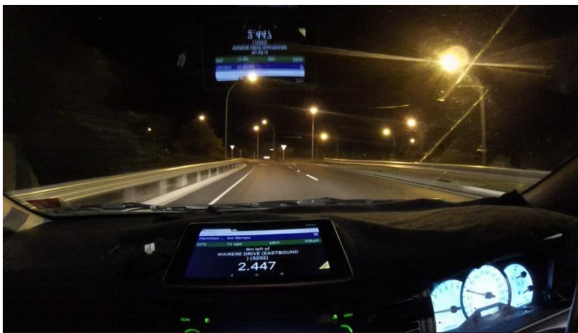
Figure 3 View from the internal video camera with vehicle location displayed on the computer tablet
