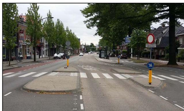
Figure 14: Central busway changes direction mid-block, Enschede, Netherlands
