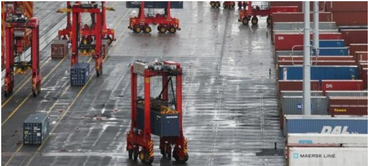
Figure 4 AutoStrad cradles at Port Botany in Sydney (Sydney Morning Herald, 2015) 6
