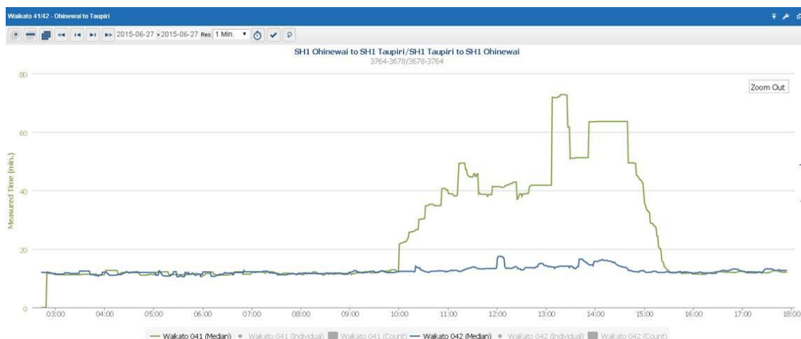
Figure 10 SH1 (Waikato) Journey Time Information from Bluetooth and Wi-Fi Data for Saturday 27th June 2015
