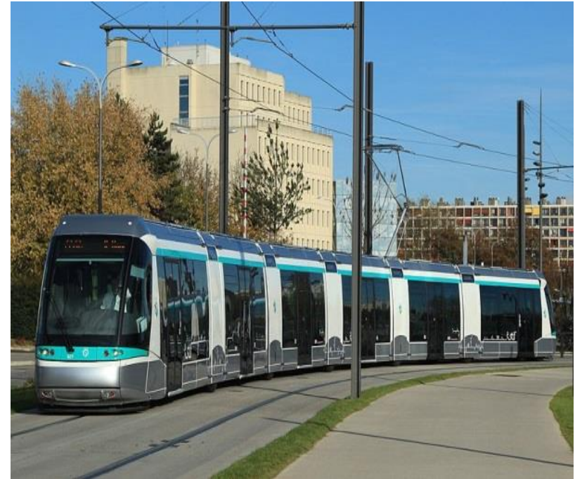
Translohr STE6 Rail Guided Electric Bus (Paris Line 6)
