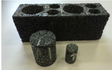
Figure 4: Cored PReSBOX sample with 100mm and 50mm specimens
