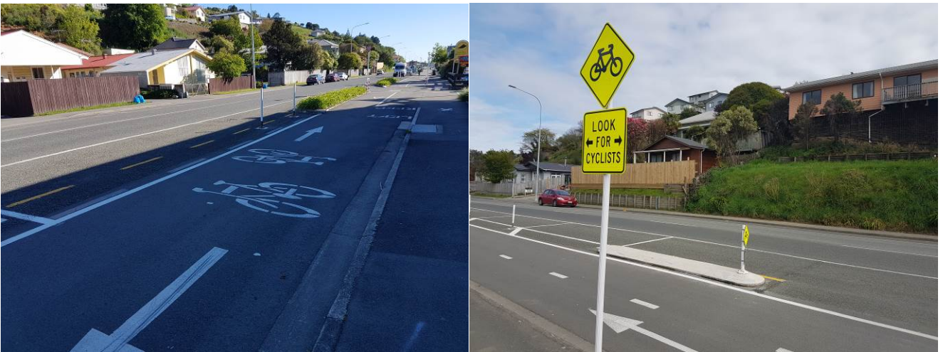
Photograph 3 Commercial access pavement markings and signage
