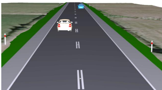
Figure 5: Proposed treatments: (Experimental) Centre line marking on straights – Rural Arterial
