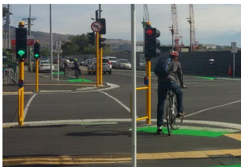
Figure 10: Directional cycle signals on Antigua St north approach to St Asaph St
